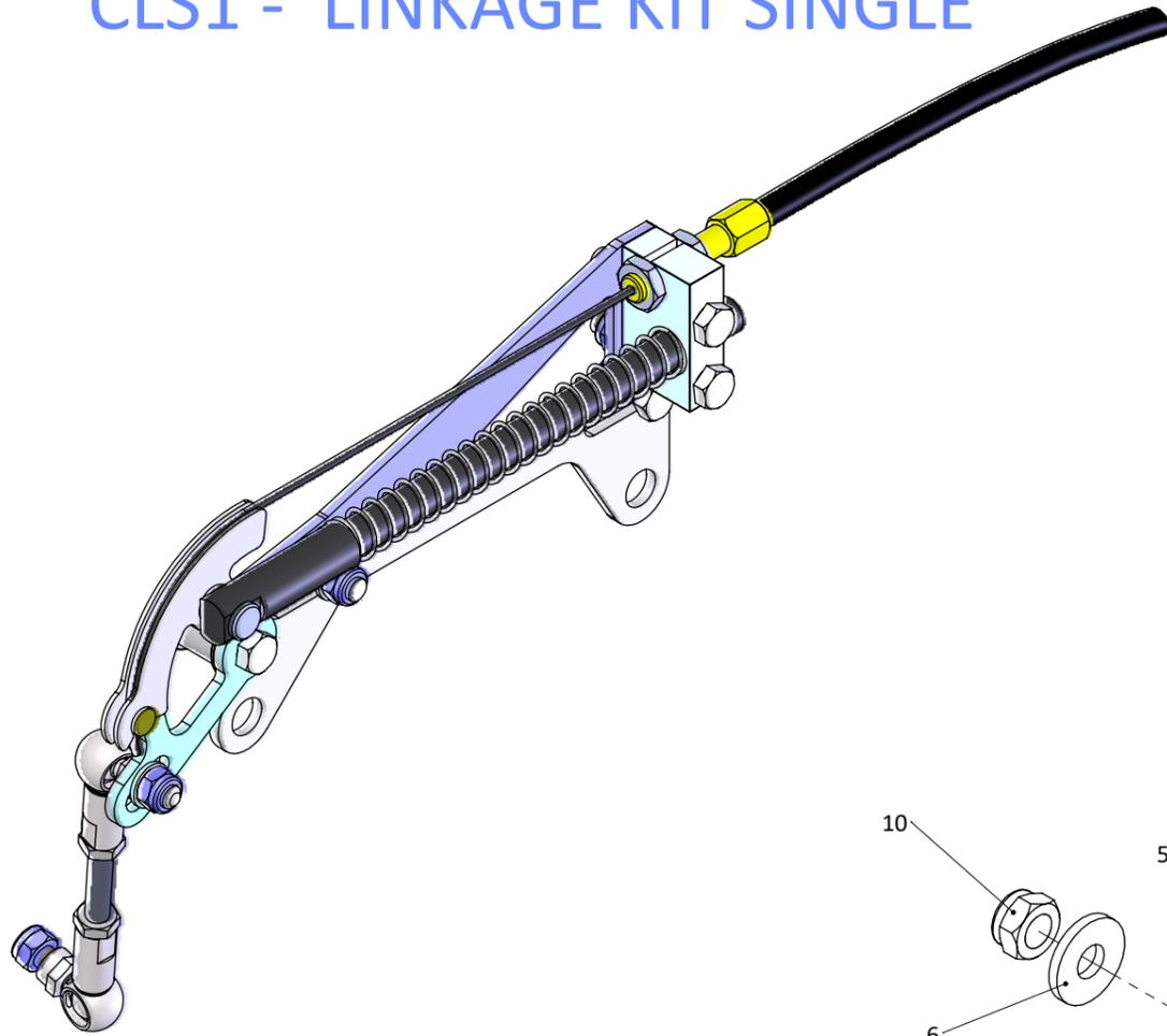
Parts may be mirrored or moved to the opposite sides of their mountings to change the axial position of the final output.
